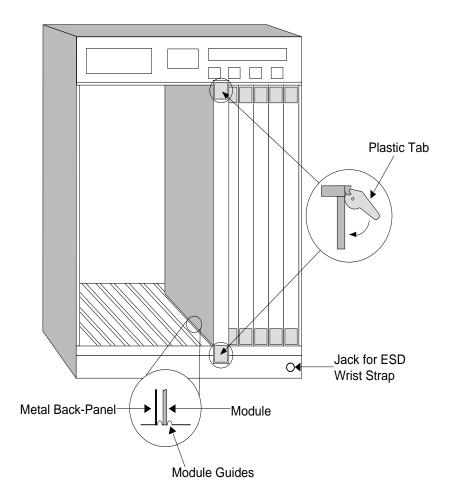
Figure 2-1. Installing the 9E106-06 Module
